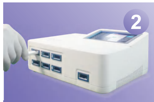
2 Put the test strip into the incubation channel.
