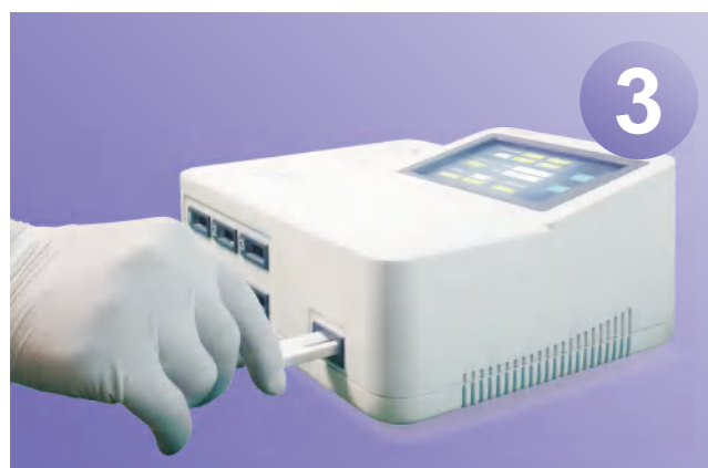
3 After incubation, put the test strip into the test channel.
